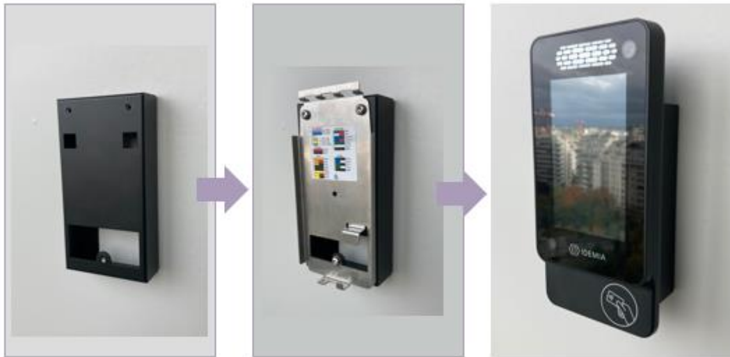
Mounting of the wall mount with 3 included screws
