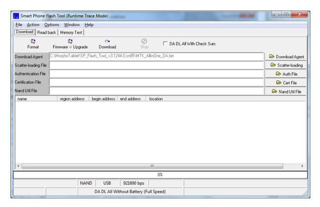
Click on **Scatter-loading** button and select the file **MT6577\_Android\_scatter\_emmc.txt** file in the Firmware release which you want to load. For the release version 01.00.102, the file is located into:
